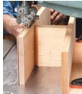
▲ A single-point fence allows you to change the feed angle to compensate for blade drift.
