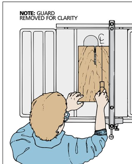
**Preventing Pull.** To prevent a workpiece from pulling away from the rip fence during a cut, center the push block between the blade and fence. Then apply gentle pressure toward the fence throughout the cut.
