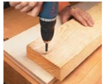
▲ *The fastest way to get a straight edge on rough lumber is to fasten it to a carrier board.*
