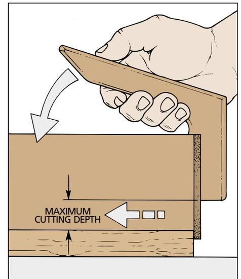
**Two-Way Fence.** The angled handle not only provides a comfortable grip for your hand, but also force in two directions. It allows you to push straight ahead and also press the workpiece down (to prevent chattering).
