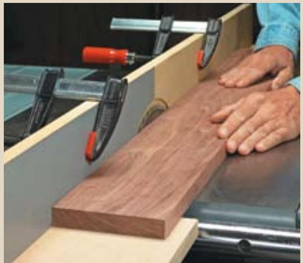
▲ Using a table saw as a jointer takes a minimum amount of setup. An auxiliary fence with laminate attached can be clamped to the rip fence.
