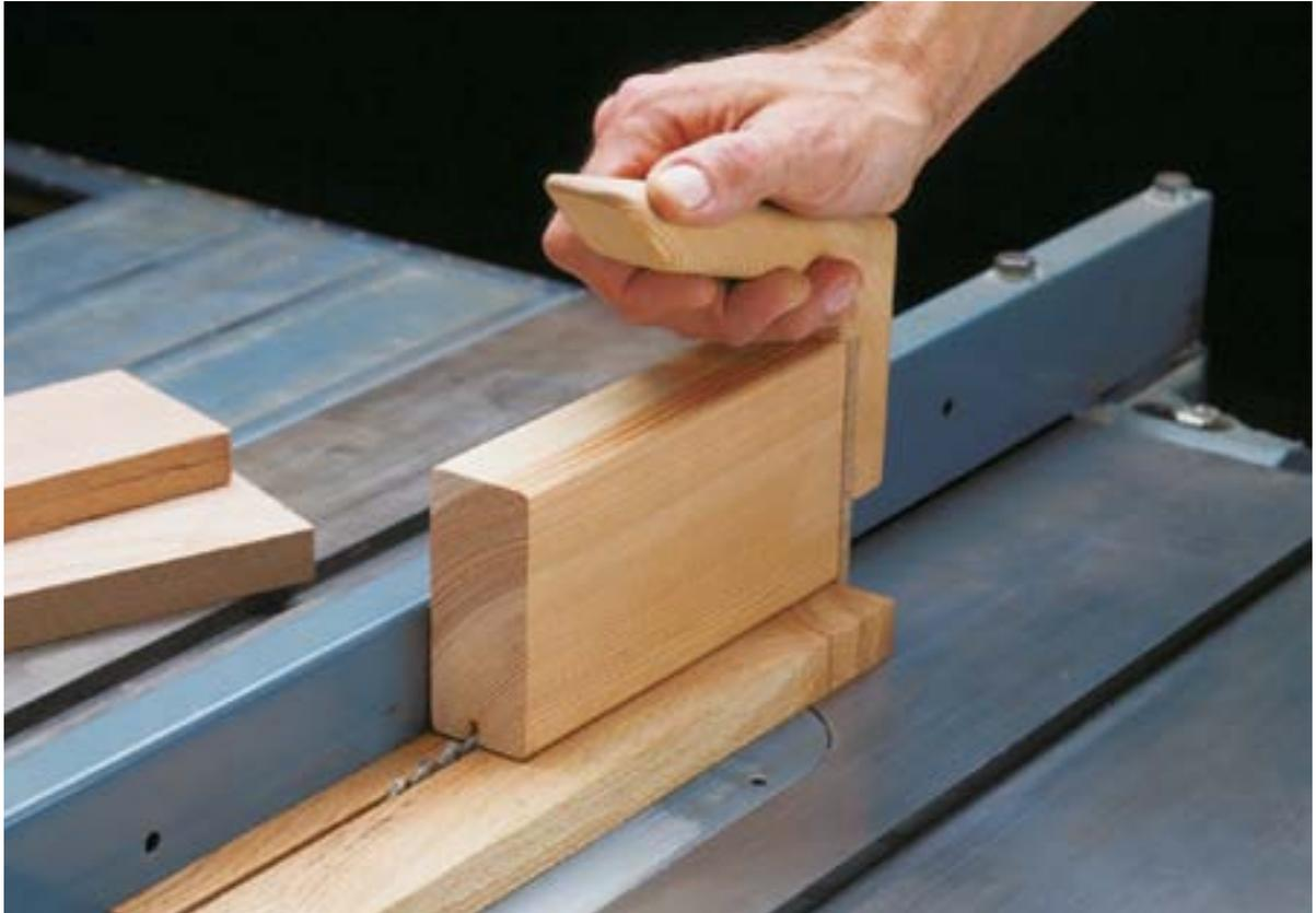
Using a push block on a table saw is just good sense: it keeps the workpiece under control and it provides a protective barrier between your hand and the saw blade.
