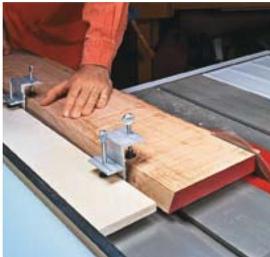
▲ Jointing clamps are made specifically for obtaining a straight edge on rough lumber. They clamp to the workpiece and a guide board.
