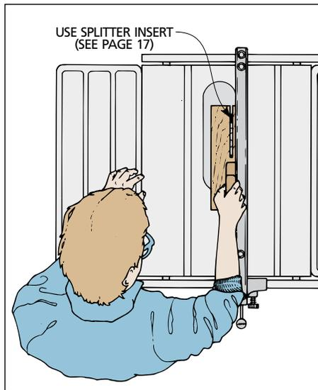
**Ripping Thin Strips.** This push block can be very helpful when ripping thin strips on the table saw. The body keeps the thin strip steady, while the heel pushes the thin strip smoothly through the blade without kickback.
